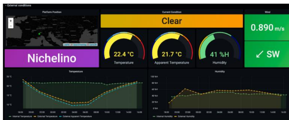
Figure 11. Sample view of the third dashboard section: external conditions.
