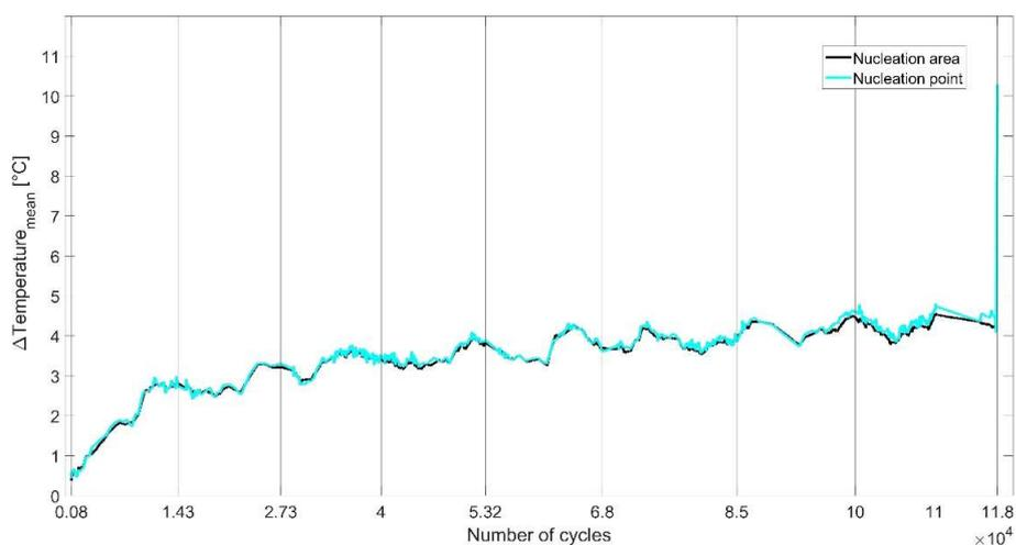
Figure 7. Gear 1 thermal profiles.
