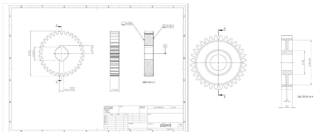
**Figure 1.** Technical drawings of Gear 1 and Gear 2.
