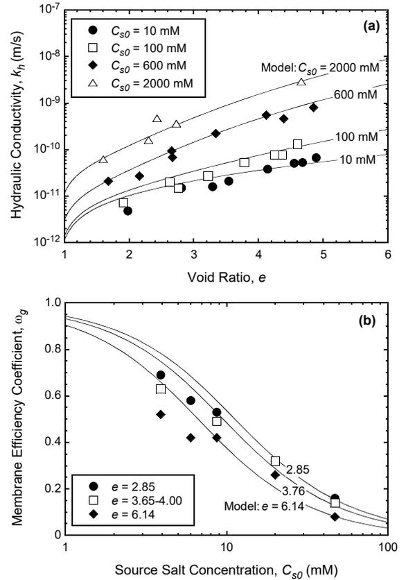
Fig. 3. Comparison of experimental data and model predictions for sodium bentonite GCLs based on fabric boundary surface parameters  $N_{i,AV0} = 2.85$ ,  $\alpha = 8.49$ , and  $\beta = 9.39$ : (a) hydraulic conductivity to NaCl solutions (Petrov and Rowe, 1997); (b) global membrane efficiency coefficients for KCl solutions (Malusis and Shackelford, 2002a).
