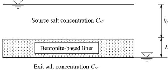
Fig. 2. Reference scenario for the steady-state analysis.
