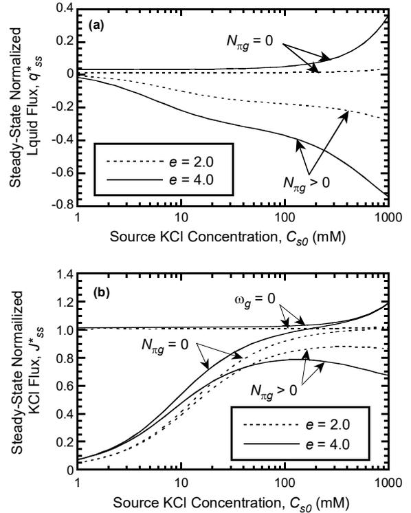
Fig. 7. Predictions of (a) steady-state normalized liquid flux,  $q_{ss}^*$ , and (b) steady-state normalized salt (KCl) flux,  $J_{ss}^*$ , as a function of source concentration and void ratio.
