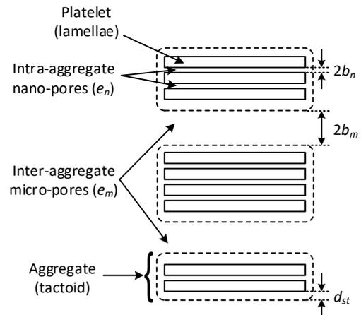
Fig. 1. Conceptual view of montmorillonite fabric showing clay platelets (lamellae) aggregated into three tactoids arranged in parallel (redrawn after Manassero, 2020;  $b_n$  = half-distance between platelets,  $b_m$  = half-distance between adjacent tactoids,  $d_{st}$  = thickness of Stern layer surrounding each tactoid).
