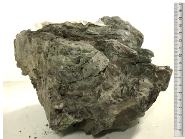
Figure 2. A typical irregular mélange lump extracted manually.
