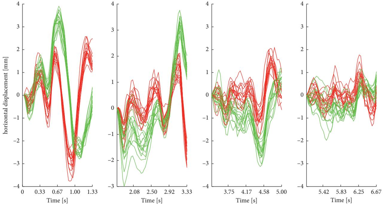
FIGURE 12: Four sections of the extracted displacement time histories ( $\alpha = 4$ ; red: 15 output channels corresponding to the left building; green: 15 output channels corresponding to the right building).
