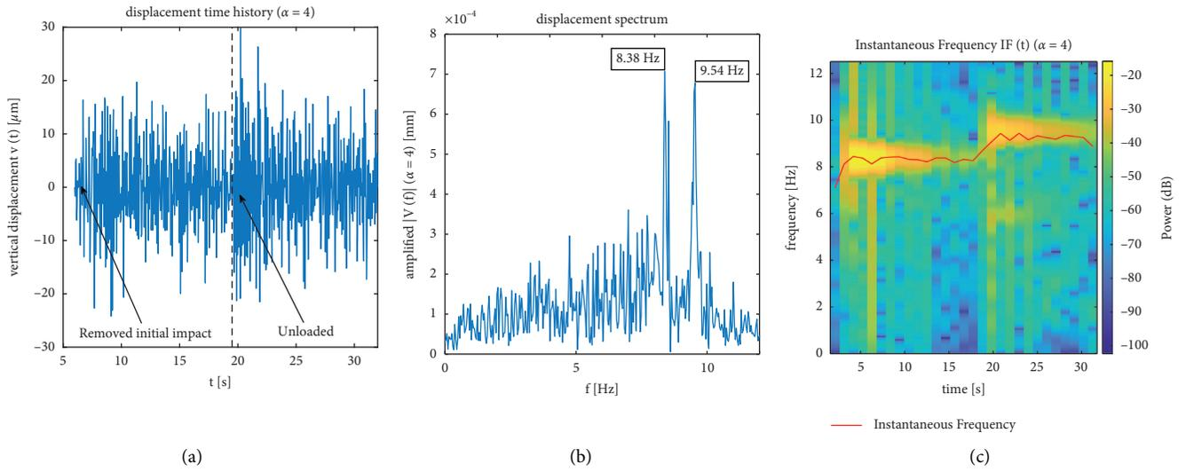
FIGURE 8: Results from the cantilevered beam (3rd experimental setup, mid-length virtual sensor,  $\alpha = 4$ ). (a) the extracted time history; (b) the Fourier Transform of the same; (c) the corresponding time-frequency plot and the instantaneous frequency (IF).
