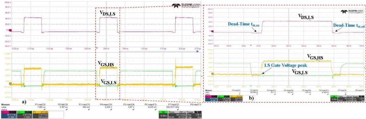
Fig. 6 a) the steady-state waveforms at 500kHz, I_L=10A and V_{DC}=48V . b) zoomed view of a single switching cycle, with the dead time highlighted. V_{DS,LS}=20V/div , V_{GS,LS}=V_{GS,HS}= 2V/div , a) t=500ns , b) t=100ns .
