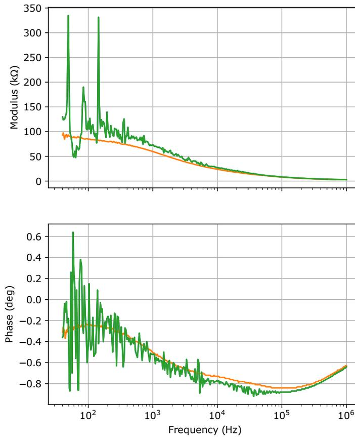
Figure 3: Impedance modulus and phase of the same plant when the watermark sensor is connected to the reading circuitry (green lines) and with the relay used to disconnect it (orange lines). The measurements were taken a few minutes away from each other in order to have similar conditions.
