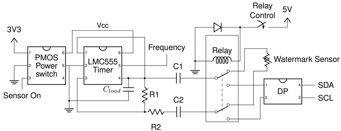
Figure 2: Schematic of the watermark sensor reading circuitry
