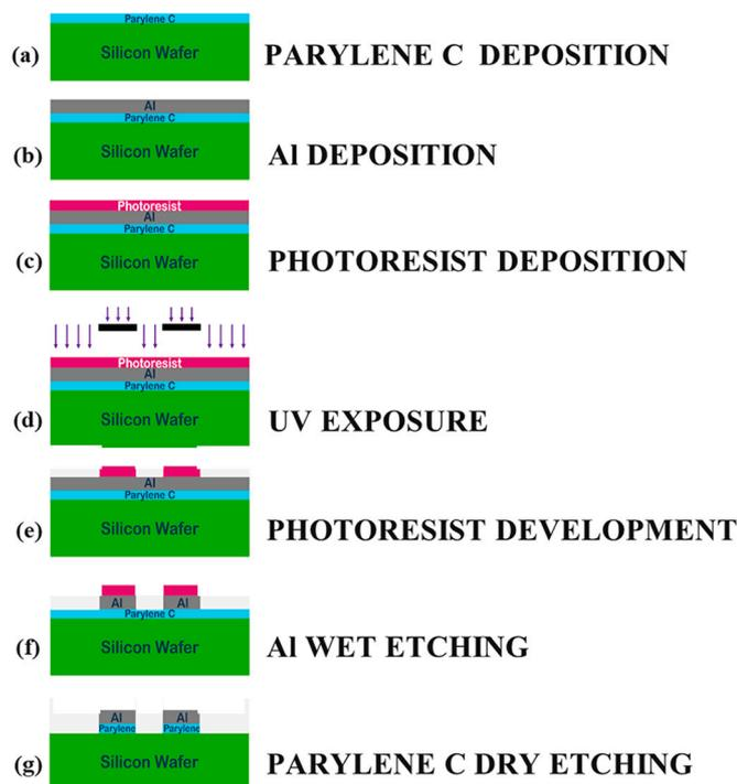
**Fig. 3.** Schematic representation of the parylene C microstencils fabrication process: (a) Parylene C deposition on top of the substrate, (b) Al thin film deposition; (c) Photoresist deposition; (d) UV exposure; (e) Photoresist development; (f) Al wet etching; (g) Parylene C dry etching.
