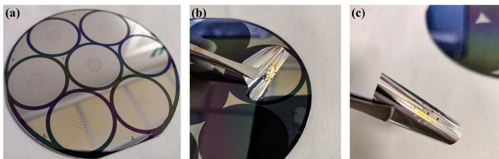
**Fig. 4.** Images of the peeling off process: (a) Single wafer with seven Parylene C shadow masks at the end of the fabrication process; (b) Single microstencil is lifted-off from the silicon wafer; (c) Flexible ready to use shadow mask.
