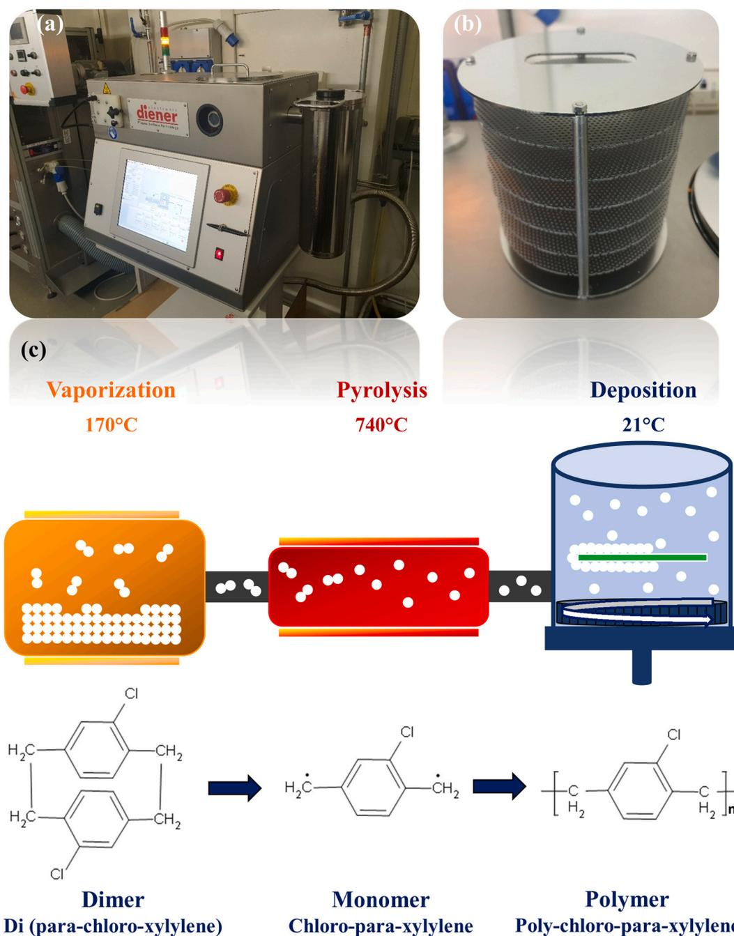
**Fig. 1.** (a) Diener Electronic – Parylene P6 deposition system (b) Multi-stage frame for samples loading into the deposition chamber (c) Sketch of the parylene C coating process, divided in three phases: the vaporization; the pyrolysis; and the deposition step. Beneath, the parylene C chemical formula from the dimeric powder to the deposited polymer.
