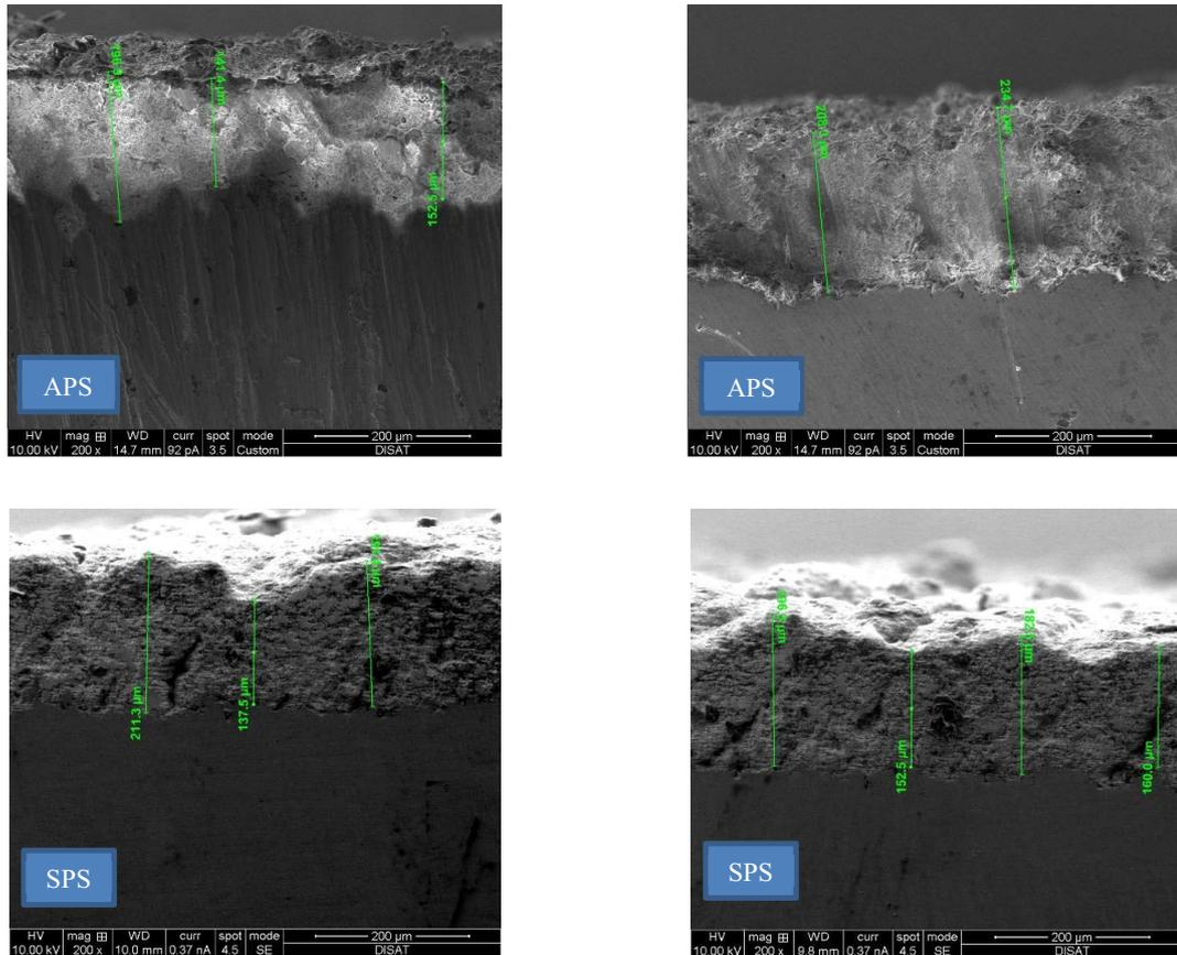
**Figure 2.** SEM results of SPS and APS specimens.
