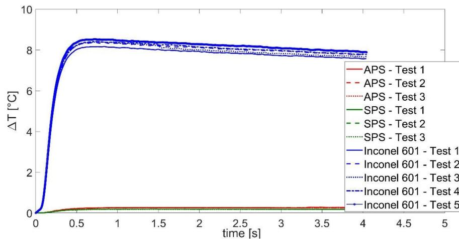
**Figure 5.** Relative temperature  $\Delta T$  of each specimen.
