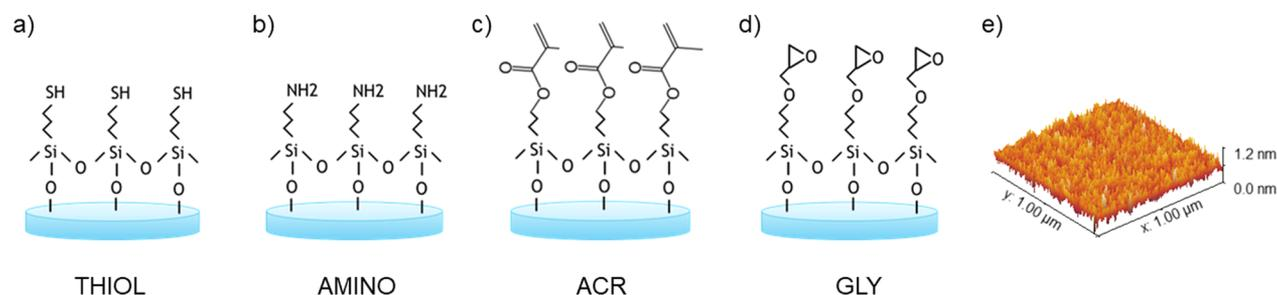
**Figure 1.** Overview of the surface chemistries employed in the present study: (a) THIOL, (b) AMINO, (c) ACR, and (d) GLY SAMs. (e) Representative topography of a glass surface that has been functionalized with THIOL SAM.
