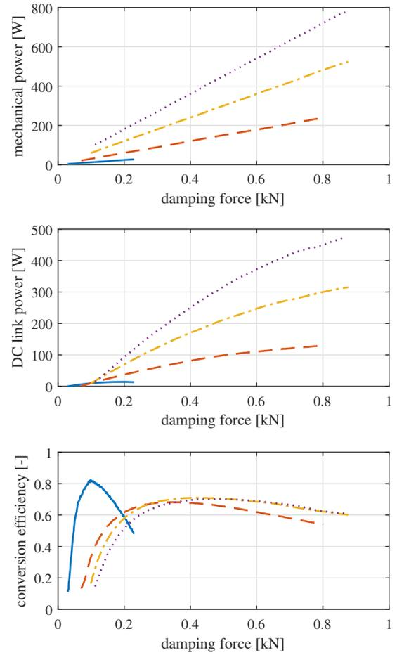
**Figure 11.** Rotary electromechanical damper prototype test results. Power contributions and conversion efficiency at constant speed of the prototype input shaft: 10 (solid), 25 (dashed), 50 (dash-dotted) and 75 rpm (dotted).
