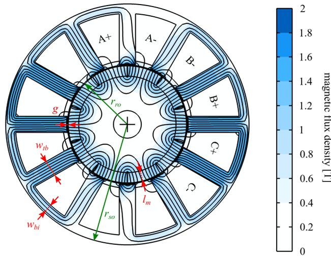
**Figure 3.** Electric machine cross section. The colour map indicates the flux density norm distribution, whereas the contour lines denote the out-of-plane magnetic vector potential. Letters in the slots indicate the winding layout for the three phases (A,B,C). Dimensions are reported in table 2.
