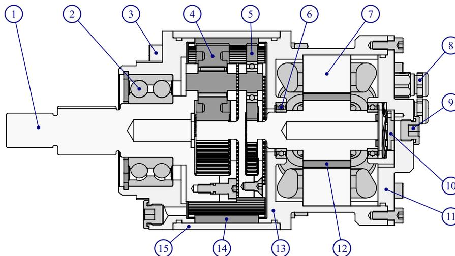
**Figure 5.** Rotary electromechanical damper actuation unit. (1) input shaft; (2) input bearing; (3) gearbox cover; (4) first stage assembly; (5) second stage assembly; (6) motor ball bearing [ $\times 2$ ]; (7) stator assembly; (8) cable gland [ $\times 4$ ]; (9) drain cap [ $\times 2$ ]; (10) position sensor; (11) motor cover; (12) rotor assembly; (13) motor casing; (14) outer ring gear; (15) gearbox casing.
