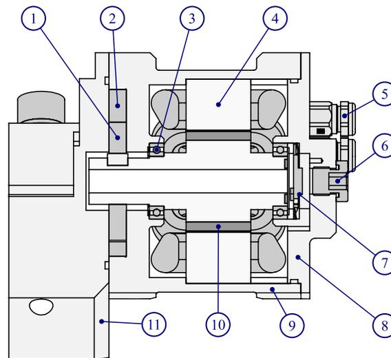
**Figure 4.** Electro-hydrostatic damper actuation unit. (1) gerotor inner gear; (2) gerotor outer gear; (3) motor ball bearing [ $\times 2$ ]; (4) stator assembly; (5) cable gland [ $\times 4$ ]; (6) drain cap; (7) position sensor; (8) motor cover; (9) casing; (10) rotor assembly; (11) manifold.
