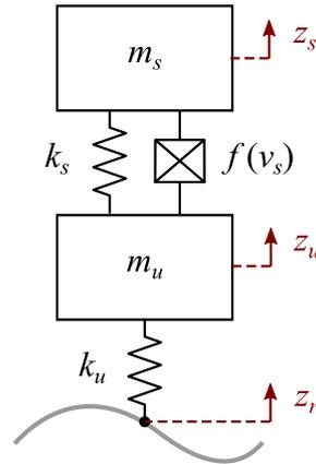
**Figure 2.** Quarter-car model to evaluate damper duty cycle.
