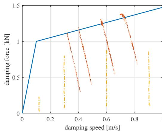
**Figure 12.** Characterised points in the force-speed plane for the electro-hydrostatic (dotted) and the rotary electromechanical (dash-dotted) prototypes. The target maximum damping characteristic (solid) is shown for comparison purposes.
