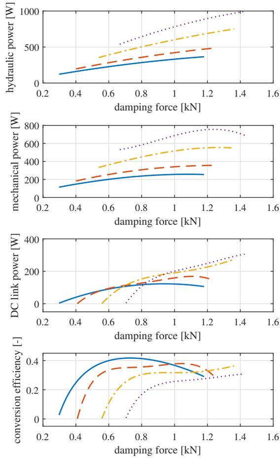
**Figure 10.** Electro-hydrostatic damper prototype test results. Power contributions and conversion efficiency at constant speed of the driving motor and pump: 1 (solid), 1.2 (dashed), 1.6 (dash-dotted) and 2krpm (dotted).
