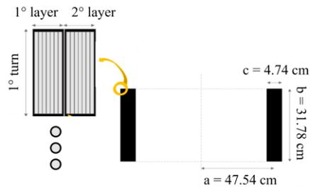
Figure 2. Basic design geometry of the SMES module.
