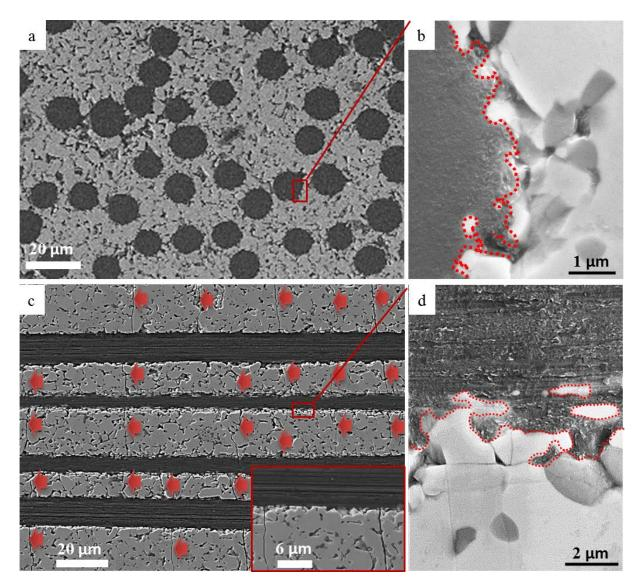
Fig. 2. SEM micrographs of the polished cross section of the UHTCMC based on pitch-derived carbon fibers and  $ZrB_2/SiC$  matrix along (a,b) the transverse direction, and (c,d) longitudinal direction. The dotted lines highlight the jagged fiber/matrix interface. The arrows point the presence of cracks in the matrix. The inset in © shows a detail of the cracked matrix.
