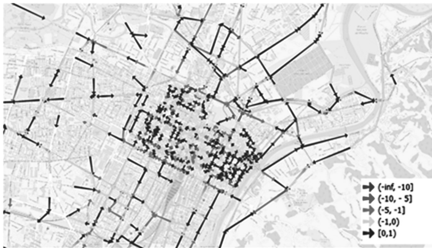
Fig. 8 – Value of the mean indicator computed for all the arcs of the road network, zoom in the Turin city centre (Reproduced from Pirra and Diana (2019) under the licence https://creativecommons.org/licenses/by/4.0/legalcode ).
