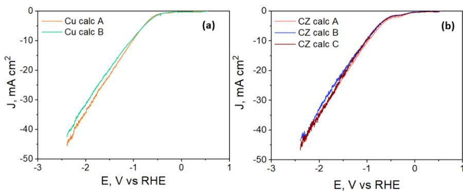
Figure S1. Linear sweep voltammetry (LSV) for Cu calc (a) and CZ calc (b) catalysts, deposited in a carbon paper support. The test was carried out in a CO<sub>2</sub>-purged 0.1 M KHCO<sub>3</sub> electrolyte (scan rate: 5 mV s<sup>-1</sup>) with a catalyst loading of 1.5 mg cm<sup>-2</sup> in a three-electrodes electrochemical cell.
