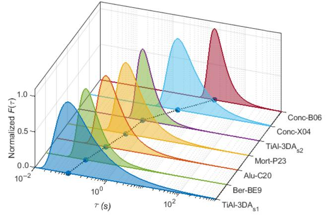
FIG. 4. Normalized representative distributions of all the investigated materials, plotted as a function of increasing peak position. The dashed line connects the projection of the peak positions on the zero-amplitude plane.
