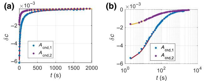
FIG. 1. Evolution of the relative velocity variation in the sample Conc-B06, during the relaxation process for two different conditioning amplitudes. (a) Linear time scale. (b) Logarithmic time scale.
