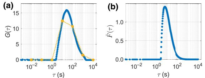
FIG. 2. (a) Discrete distribution,  $G(\tau)$  in the logarithmic time scale obtained by using a basis of seven exponentials (yellow symbols). Repeating the fitting by shifting the  $B_1$  (initial value for the basis), we obtain a continuous distribution (blue symbols). (b) Estimation of the distribution  $\hat{F}(\tau)$  in the linear time scale, inferred from  $G(\tau)$ .
