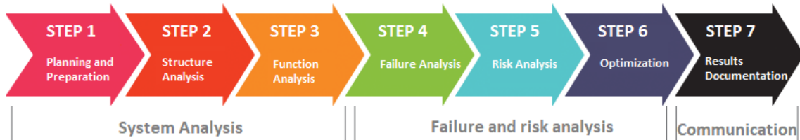
Figure 2.13: The 7 steps described by the AIAG and VDA FMEA manual. Figure from [5].
