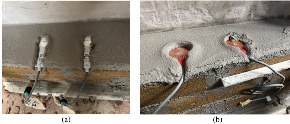
Figure 3. Installation of the sensors in the mortar bed-joints: (a) ceramic sensors; (b) capacitive sensors.
