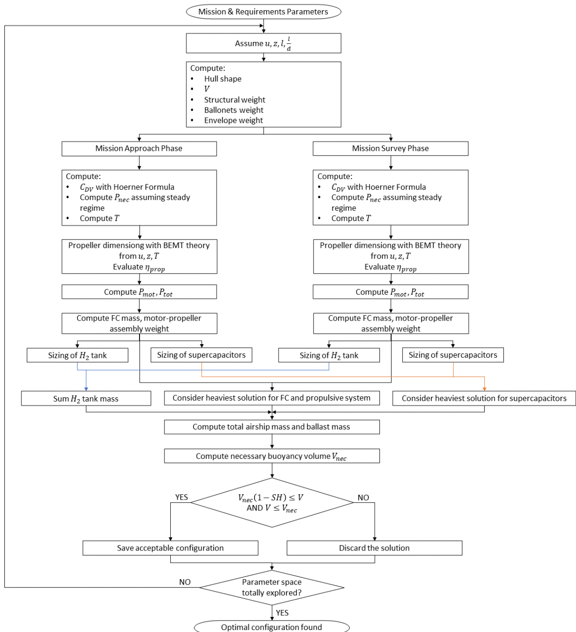
Figure 14 - Flow chart of the numerical routine.
