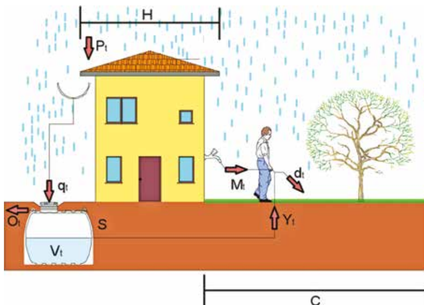
Fig. 1 – Configuration of the rainwater harvesting system.
