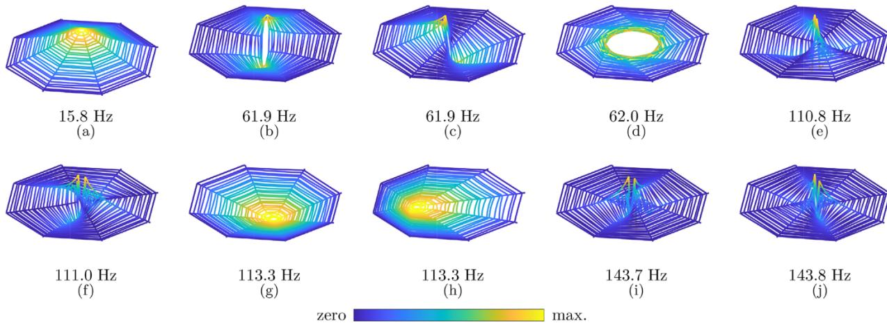
**Figure 4.** Modes of vibration and natural frequencies considering only the orb web and spider masses. Mode (a) is a transverse displacement mode; modes (b) and (c) represent bending modes; mode (d) is a torsional mode; modes (e), (f), (i), and (j) are second order-like bending modes, and modes (g) and (h) are in-plane translational modes. Colors indicate zero and maximum values of absolute displacements.
