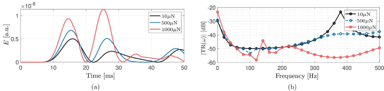
**Figure 12.** Effects of material nonlinearity. a) The effects of nonlinearity on the energy at the orb web center output nodes substantially increase for sufficiently large force values. b) For sufficiently large force values, the frequency response presents a larger decrease up to 120 Hz, after which it maintains a relatively uniform response up to 500 Hz.
