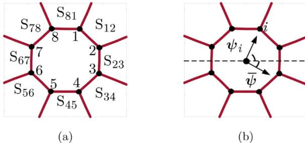
**Figure 13.** Quantities used in prey location estimation. a) Sections defined as regions between two adjacent output nodes and their corresponding radial threads. b) Heading angle associated with the  $i$ th output node,  $\psi_i$ , and estimated heading angle,  $\bar{\psi}$ .
