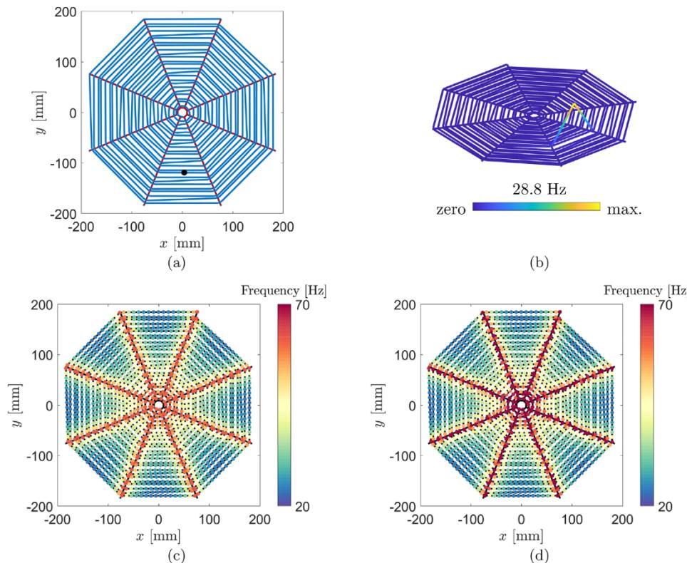
**Figure 5.** Locally resonant out-of-plane transverse mode and frequencies due to prey impact. a) An example of prey location with its b) corresponding locally resonant out-of-plane normal mode indicating a frequency of 28.8 Hz. Colors indicate zero and maximum values of absolute displacements. c) Colormap indicating impact points with corresponding resonant frequencies on the orb web domain for a radial thread pre-stress of 100 MPa. d) Same as (c), but with a prestress of 150 MPa.
