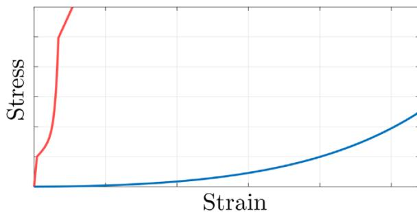
**Figure 2.** Stress–strain relations for (■) dragline and (■) viscid silk threads.
