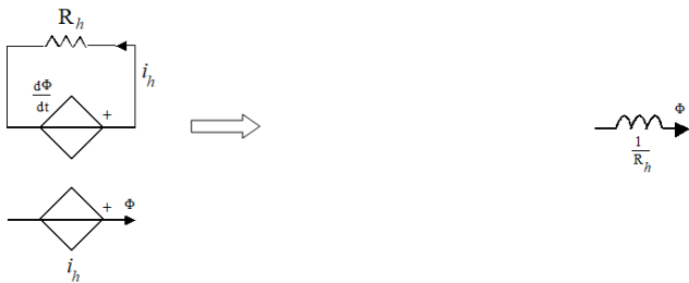
Figure 7. Coupling between magnetic and eddy current domain
