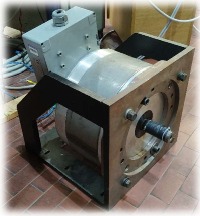
Fig. 6. Automotive inductor motor used for the tests.
