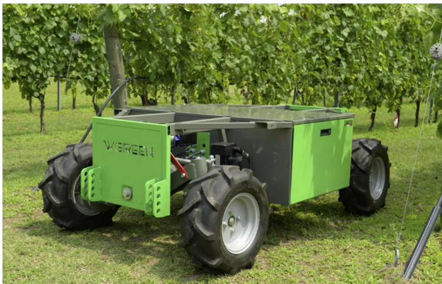
Fig. 3 – The 4WS UGV designed and developed by the Department of Agricultural, Forest and Food Sciences (DiSAFA) of University of Turin, Italy.
