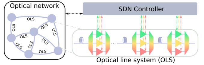
Fig. 2: Illustration of a multi-band OLS amplification.
