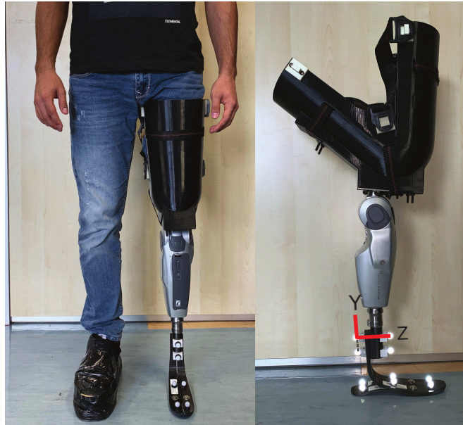
Figure 5. Test setup for ROS calculation - on the left, the healthy subject fitted with the able-bodied adapter; on the right, a sideview with the markerset highlighted. Axes of the local coordinate system (shank) are shown
