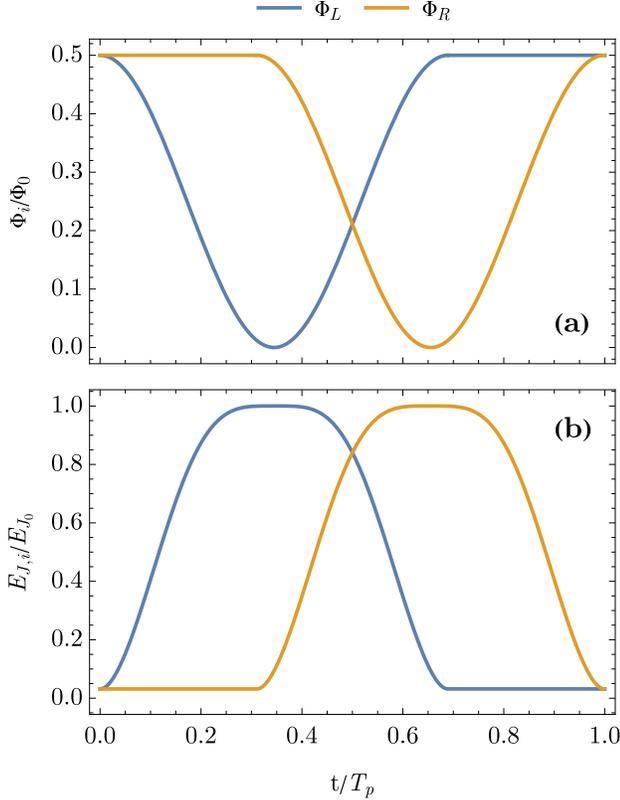
Fig. 2. (a) Magnetic flux threading the left (blue) and right (orange) loops as a function of time. The modulation of the fluxes has a cosinusoidal shape with a phase lag of  $1/3$  of a period. (b) Modulation of the Josephson energies caused by the flux modulation.  $E_{J_0}$  is the maximum value of the Josephson energy reached in one cycle.
