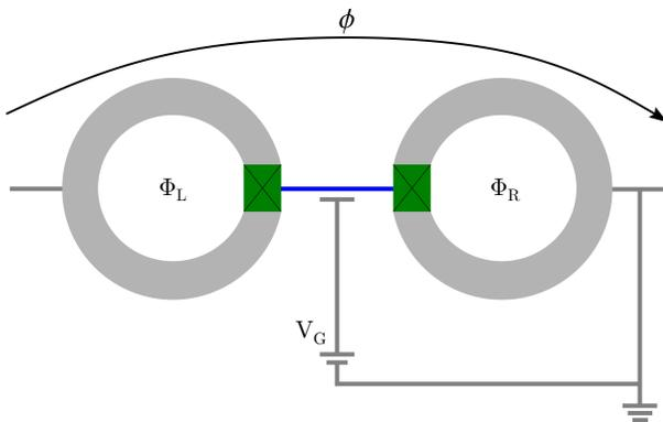
Fig. 1. Sketch of the structure of a JESP:  $\Phi_L$  and  $\Phi_R$  are the magnetic fluxes threading two superconducting loops (light grey). The (blue) island connects the two nanowires (green) and is set at the working point by the gate voltage  $V_G$ . Two Josephson junctions are formed by the nanowires plus the superconducting island. A bias phase difference  $\phi$  is kept constant at the two sides of the device.
