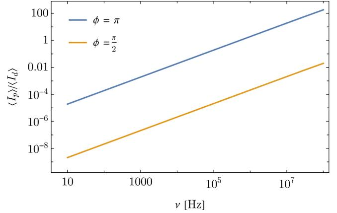
Fig. 5. Pumped current on dynamic current ratio  $\langle I_p \rangle / \langle I_d \rangle$ . The curves are calculated as a function of the pumping frequency  $\nu$  for different bias phases and  $\delta n_g = 0.03$ .
