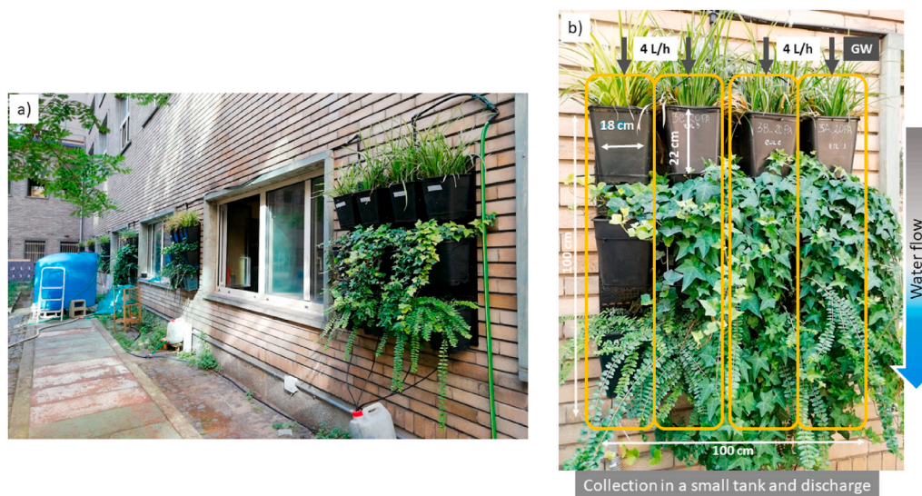
Fig. 1. a) Overview of the green wall panels; b) Detail of a modular panel. (For interpretation of the references to color in this figure legend, the reader is referred to the Web version of this article.)
