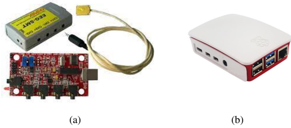
Fig. 3. BCI Equipment: a) Olimex EEG-SMT; b) Raspberry Pi4.
