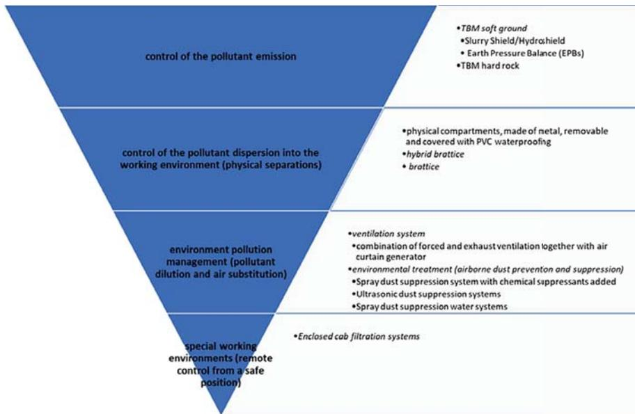
Fig. 2. Hierarchy of engineering controls proposed for tunnelling through rock masses that may contain asbestos minerals and other pollutants
