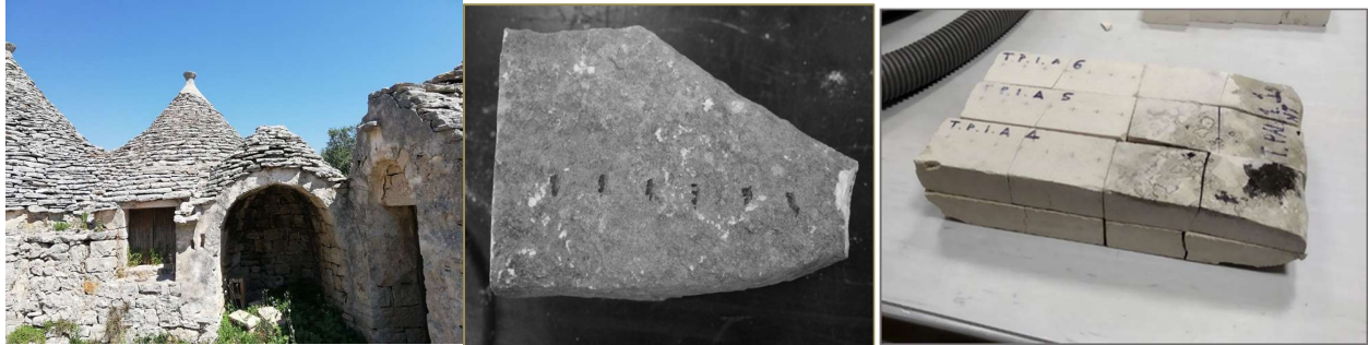
Figure 2 - The “Trullo” sampled (left) with one of the samples collected (center) and cut into specimen for the tests (right).....
