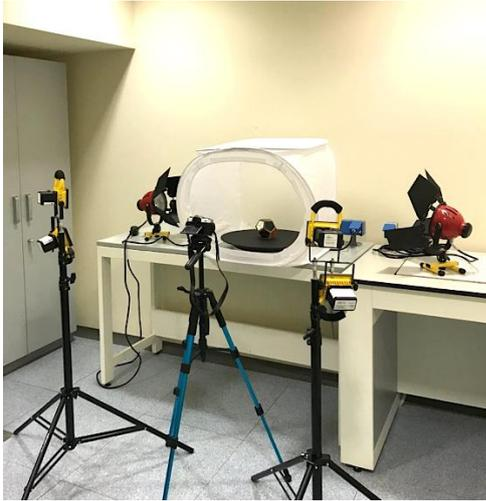
Figure 3. Photogrammetry system for multispectral images acquisitions.
