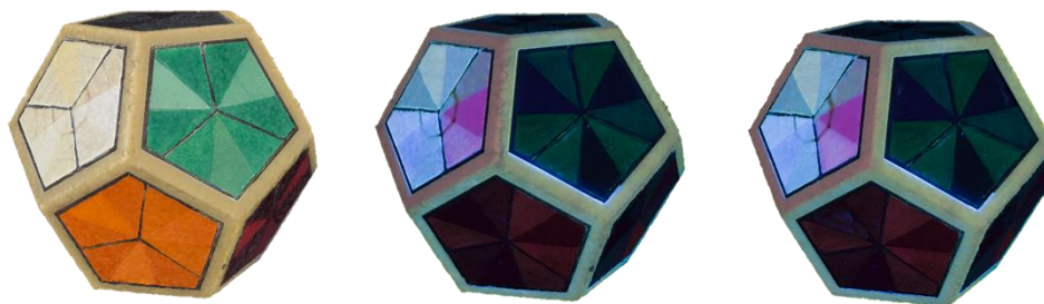
Figure 4. From left to right: 3D model from reflected VIS images; 3D model obtained after re-texturing of the reflected-VIS model with UVL images; and 3D model obtained using UVL images directly.
