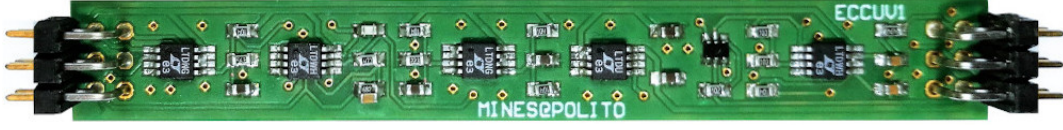
Figure 4.5: PCB implementation of QD potentiostat with COTS components; the electrochemical cell connected on pin on the left, and power supply, PWM, and QDE on the right. Adapted with permission from [102]. © 2019 IEEE
