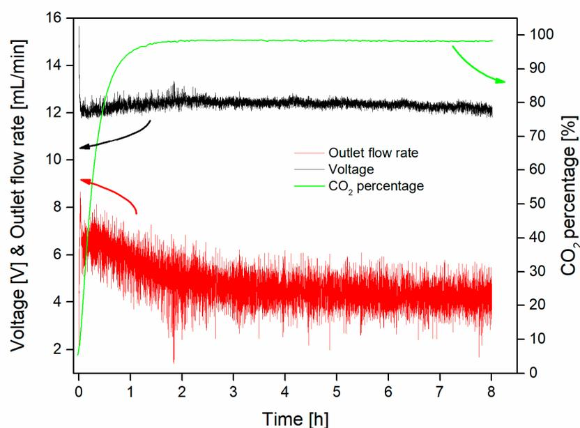
**Figure 7.** Measured voltage (left axis), CO<sub>2</sub> outlet flow rate, and purity of CO<sub>2</sub> in the outlet gas (right axis) during the stability test of eight hours (experimental conditions:  $Q_{\text{inlet}} = 20$  mL/min,  $Q_{\text{pump}} = 1$  mL/min,  $J = 100$  mA/cm<sup>2</sup>, CO<sub>2</sub>/N<sub>2</sub> ratio = 100%/0%).
