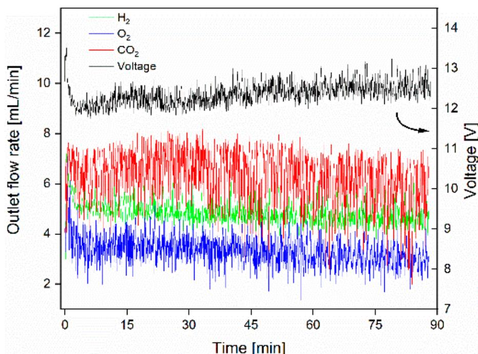
**Figure 1.**  $\text{CO}_2$ ,  $\text{O}_2$  and  $\text{H}_2$  outlet flows (left axis) and measured voltage (right axis) in a typical experiment carried out with the capture and release unit (experimental conditions:  $J = 100 \text{ mA/cm}^2$ ,  $Q_{\text{inlet}} = 20 \text{ mL/min}$ ,  $Q_{\text{pump}} = 1 \text{ mL/min}$ ,  $\text{CO}_2/\text{N}_2$  ratio = 100%/0%).
