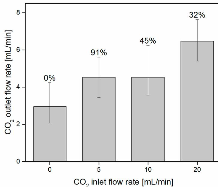
**Figure 4.** Average CO<sub>2</sub> flow for different pure CO<sub>2</sub> inlet flow rates (experimental conditions:  $J = 100 \text{ mA/cm}^2$ ,  $Q_{\text{pump}} = 1 \text{ mL/min}$ , CO<sub>2</sub>/N<sub>2</sub> ratio = 100%/0%). The values on top of the columns represent the percentage of CO<sub>2</sub> captured with respect to that provided as input.
