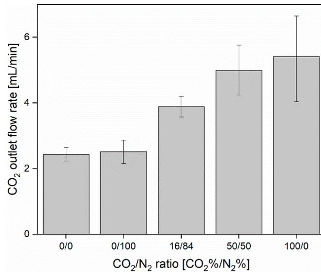
**Figure 5.** Average CO<sub>2</sub> flow for different compositions of inlet gas (experimental conditions:  $Q_{inlet} = 20$  mL/min,  $Q_{pump} = 5$  mL/min,  $J = 100$  mA/cm<sup>2</sup>).
