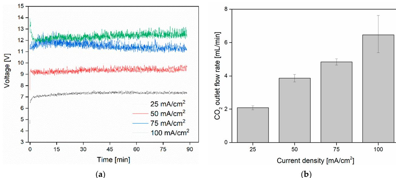
**Figure 2.** (a) Measured voltages for different applied current densities (experimental conditions:  $Q_{inlet} = 20 \text{ mL/min}$ ,  $Q_{pump} = 1 \text{ mL/min}$ ,  $\text{CO}_2/\text{N}_2$  ratio = 100%/0%). (b) Average  $\text{CO}_2$  flow for different applied current densities with the same experimental conditions.
