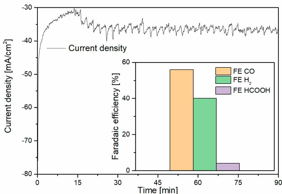
**Figure 8.** Conversion module results with an initial 50%/50% gas stream; average current density during the measure and (inset) faradaic efficiencies of the reaction products (FE = faradaic efficiency).
