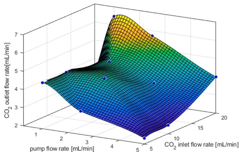
**Figure 6.** Interpolating fit of experimental CO<sub>2</sub> outlet results obtained at  $J = 100$  mA/cm<sup>2</sup> for different CO<sub>2</sub> inlet and pump flow rates. The blue points are the experimental data.
