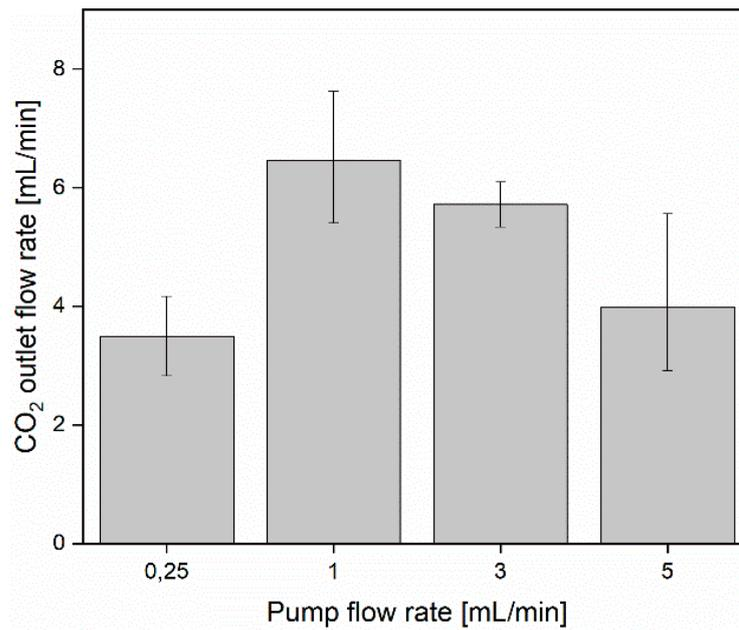
**Figure 3.** Average CO<sub>2</sub> flow for different pump flow rates (experimental conditions:  $Q_{\text{inlet}} = 20 \text{ mL/min}$ ,  $J = 100 \text{ mA/cm}^2$ , CO<sub>2</sub>/N<sub>2</sub> ratio = 100%/0%).
