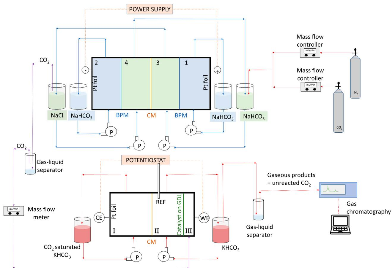
**Scheme 2.** Schematic representation of the coupling between the capture (upper reactor) and the conversion module (lower reactor). P: pump; CM: cationic membrane; BPM: bipolar membrane; CE: counter electrode; WE: working electrode; REF: reference electrode; GDL: gas diffusion layer.
