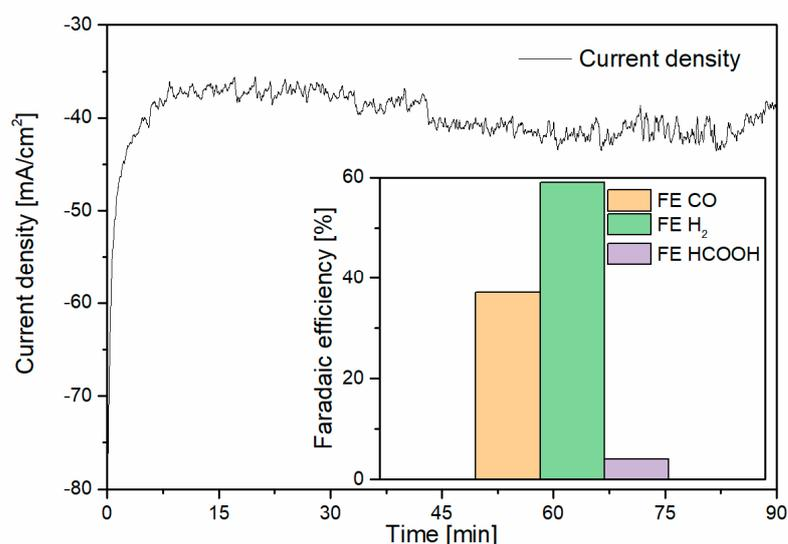
**Figure 9.** Conversion module results with an initial 16%/84% gas stream; average current density during the measure and (inset) faradaic efficiencies of the reaction products (FE = faradaic efficiency).
