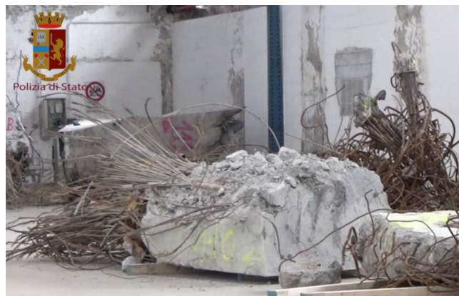
Fig. 2. (a) Triggering of the bridge collapse, which started from the failure of the SE cable-stay cross-section close to the antenna (image courtesy of Guardia di Finanza di Genova 2019); and (b) picture of the corroded strands subjected to forensic analysis (image courtesy of Polizia di Stato, republished from Bonchi (2020) with permission from Genova24).
