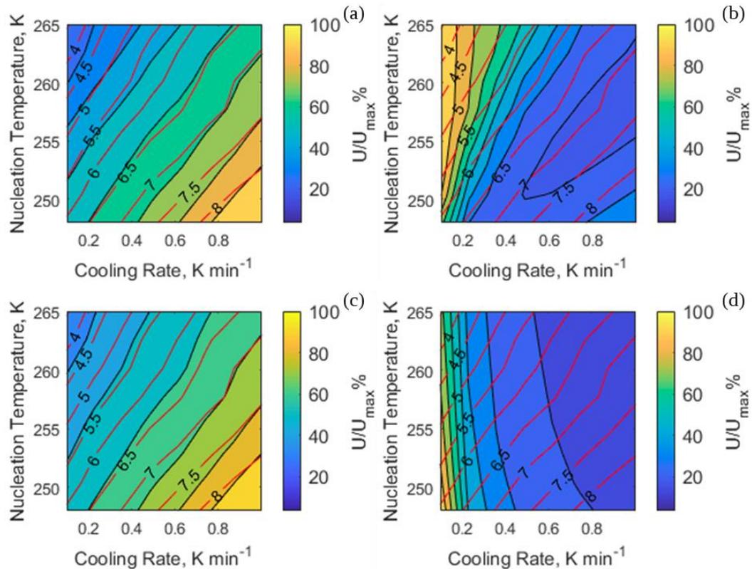
Fig. 2. Design space showing the stress for the protein (percentage of unfolded protein, normalized by its maximum value in the design space), for simulations 1 (a), 2 (b), 3 (c) and 4 (d) in Table 1. The red isocurves identify the conditions resulting in the same total extension of the ice-water surface area, reported in  $\text{dm}^2/\text{g}$  (solvent mass is used as reference) on the curves.
