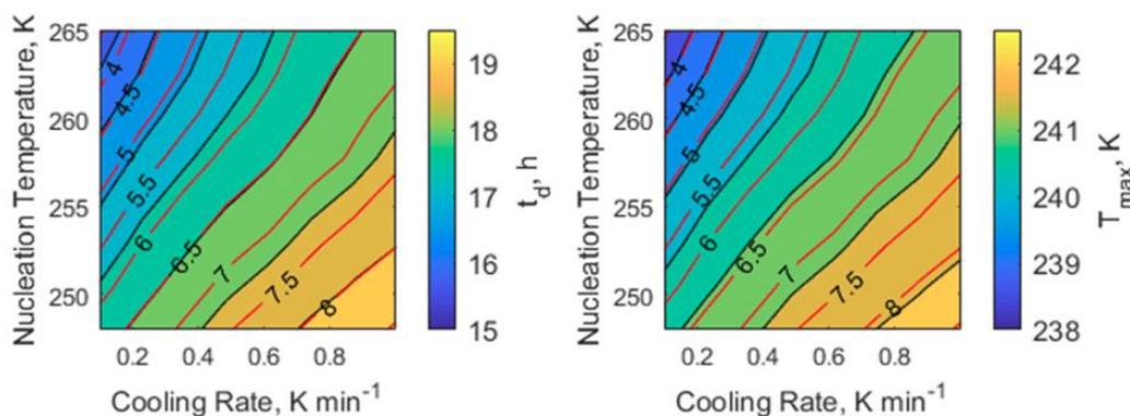
Fig. 4. Design space showing the primary drying time  $t_d$  and the maximum temperature  $T_{max}$  reached within the product. A fluid temperature and chamber pressure of 253 K and 10 Pa, respectively, have been considered for simulations of the primary drying step.
