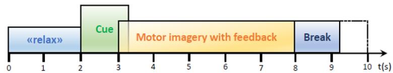
Fig. 3: Timing diagram of a single trial in the BCI experiment with neurofeedback.
