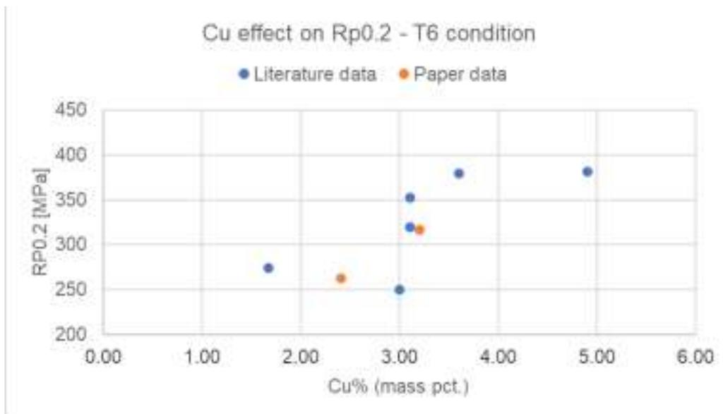
**Figure 6:** summary of the elastic limit results reported in the literature (blue dot) [6, 7, 9, 12, 16] and obtained in the present tension tests (orange dot) for AlSi9Cu3(Fe) alloy subjected to several T6 heat treatments.
