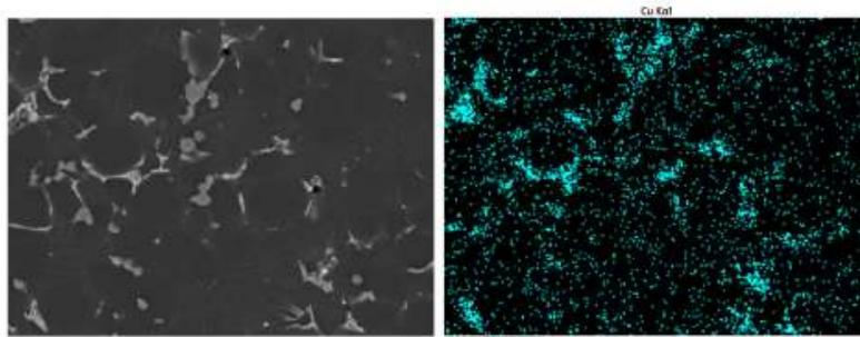
**Figure 2:** microstructure (left) and Cu composition map (right) of the same zone of a sample as cast (F temper) containing Cu=2.4%. On the left, the secondary phases (light gray) generated during the solidification process are shown. They contain Al, Si, Cu, Fe. On the right, light blue depicts the distribution of Cu in the microstructure. Single light blue points indicate Cu in solid solution, whereas light blue cluster indicate Cu containing precipitates.
