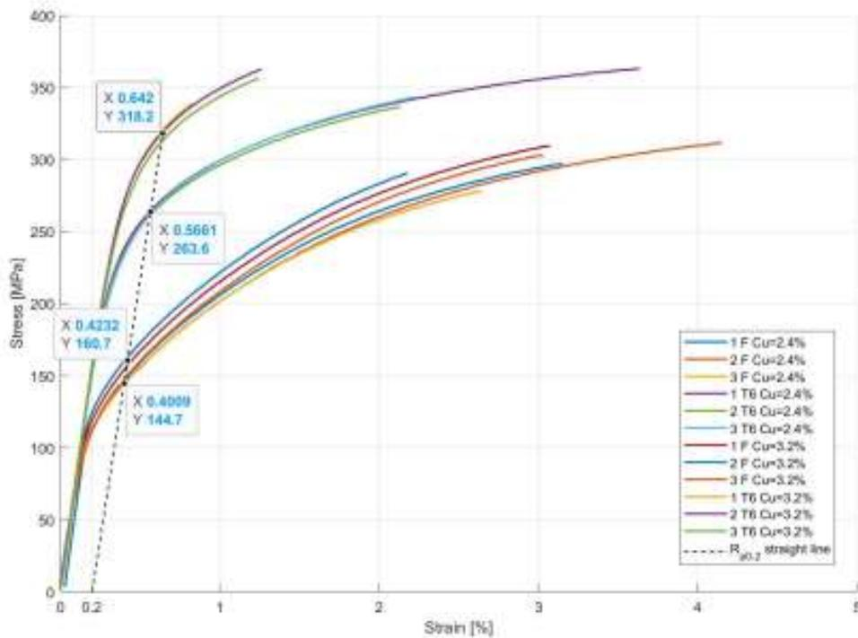
**Figure 4:** stress-strain curves obtained by tension tests. The dotted  $R_{p0.2}$  line indicated the position of the elastic limit in each curve. The letter X indicates the pct. strain at the elastic limit, the letter Y indicate the stress at the elastic limit, i.e. the conventional yield point.
