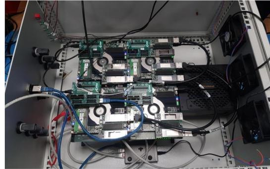
**Figure 5: Scaled-down PDPU implementation in the Test-bench**
