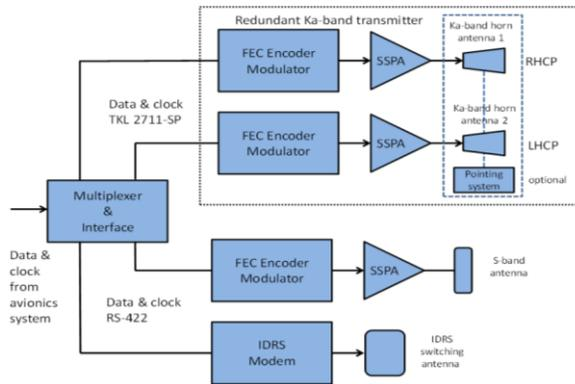
**Figure 3: EO-ALERT communications physical architecture**
