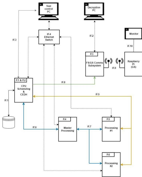
**Figure 4: Test-Bench Architecture**
