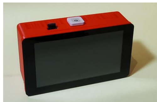
Figure 7: Handheld device and touch screen for the direct Space-to-ground decryption and visualization (used for the S-band data link transfers)
