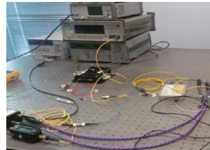
Fig.1 Optical set-up for the characterization of the photoreceiver
