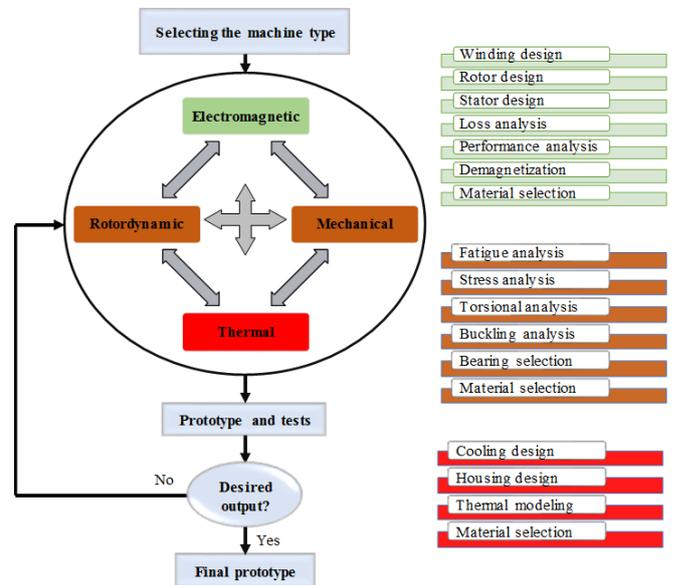
Fig. 1: Practical multiphysic design procedure of electrical machines.
