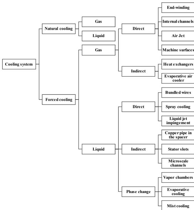
Fig. 3: Different cooling systems used in electrical machines.
