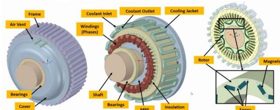
Fig. 2: Water- and air-cooled IPM machine [31].
