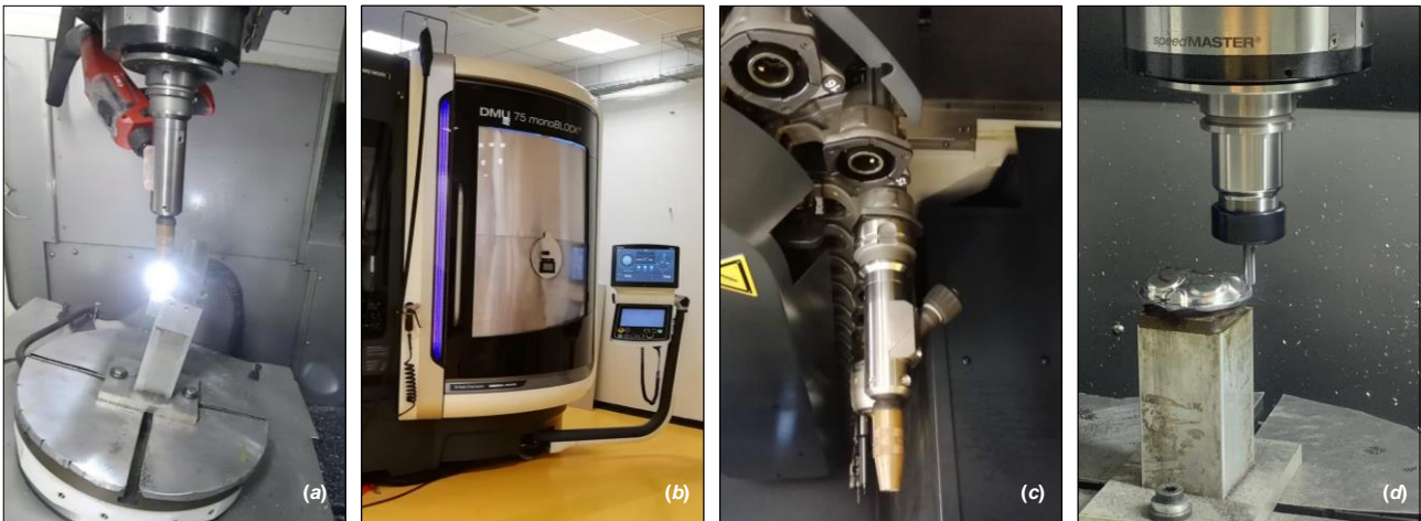
Figure 1. Experimental setup: deposition system (a), machining center (b), torch holder stored in the ATC (c), and milling head (d).
