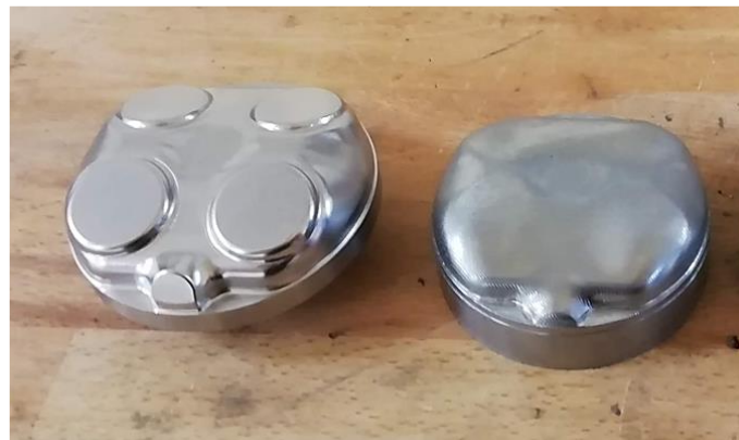
Figure 3. Result of the substrate preparation phase ( right ) with reference to the original geometry of the insert ( left ).
