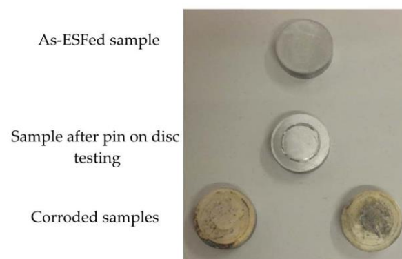
Figure 1. Macrograph of the samples employed for characterizing wear and corrosion resistance.
