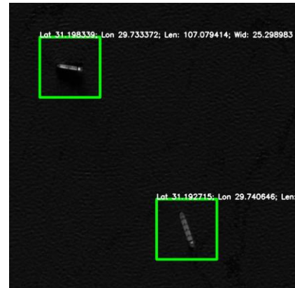
Figure 5: Ship detection algorithm results.
