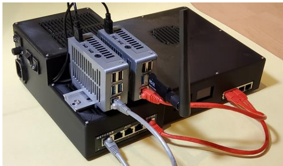
Figure 9: Communications Emulator for the complete subsystem: S-band transmitter, link controller for the iDRS transceiver, Ethernet switch and power supplies, with Ka-band emulated
