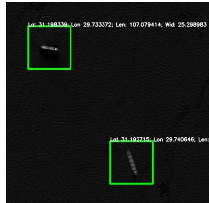
Figure 5: Ship detection algorithm results.
