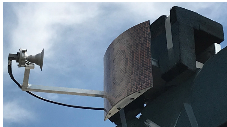
Figure 7. Photo of the entire CRA system mounted on the outdoor test range at Politecnico di Torino.
