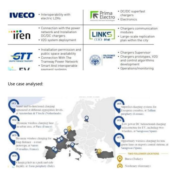
When considering the Use case n°4 expectations are to put charging hub in a park-and-ride facility in Turin adapting the tramway substation to supply the charging hub in order to use the untapped power available.
