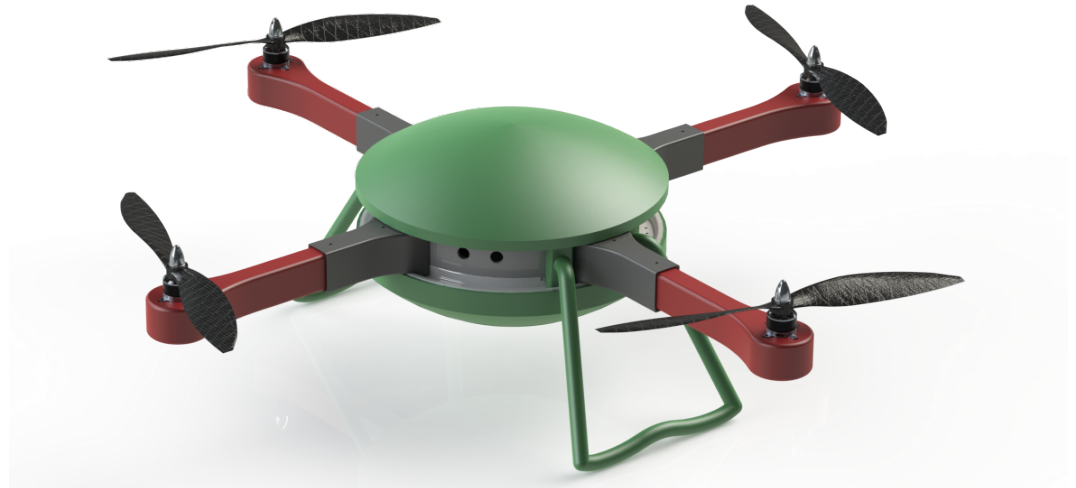
Figure 1. Graphic rendering of the PoliDrone UAV in the S4A-C configuration: four arms with a single motor/propeller each.
