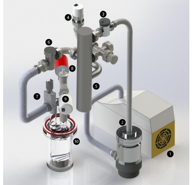
Figure 3: Launch volume/test section, subsystem 200. 1: Roots pump. 2: Turbomolecular pump. 3: Bellows sealed valve. 4: Full range pressure transducer. 5: Launch volume. 6: Bellows sealed valve. 7: Gate valve. 8-9: Capacitive pressure transducers. 10: Test section.
