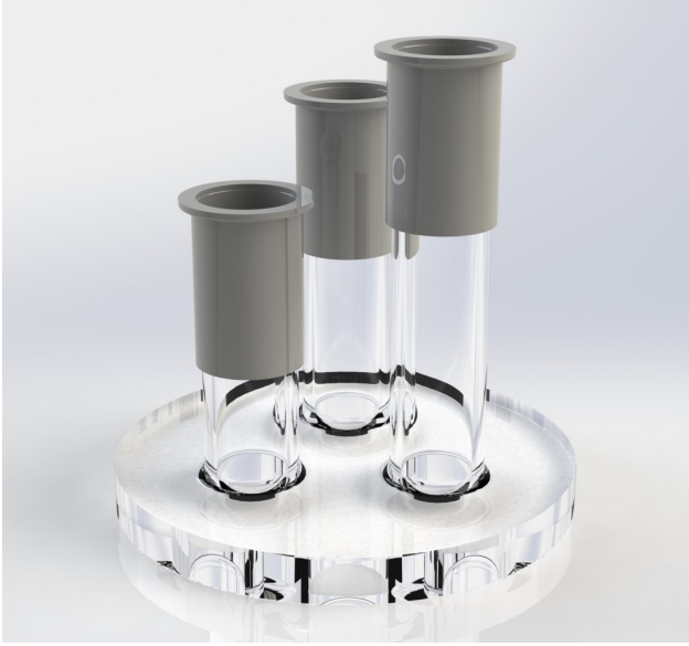
Figure 5: Upper flange with quartz-to-metal connections.
